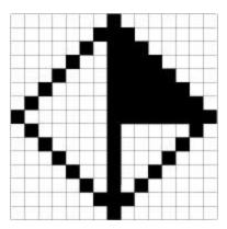
2. Convert each of the squares to either a one or a zero, where the blank boxes are zeros and the filled-in boxes are ones. Type these into a text file column by column, as shown here:
